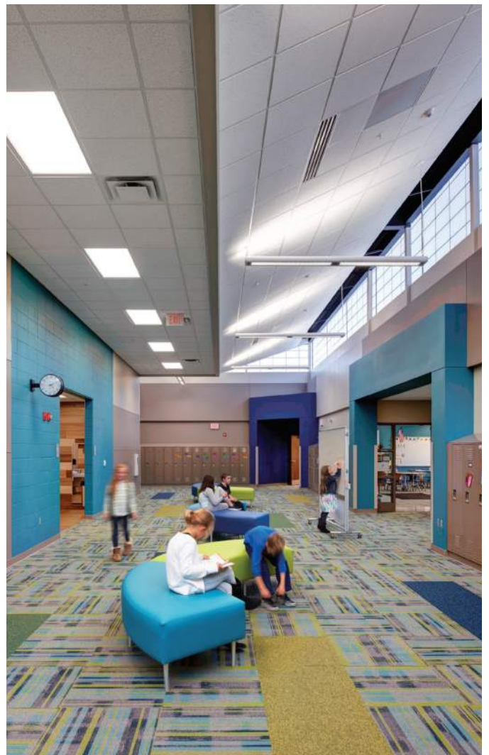
A continuous translucent panel clerestory window provides diffused natural light that brings the colors and students to life.
